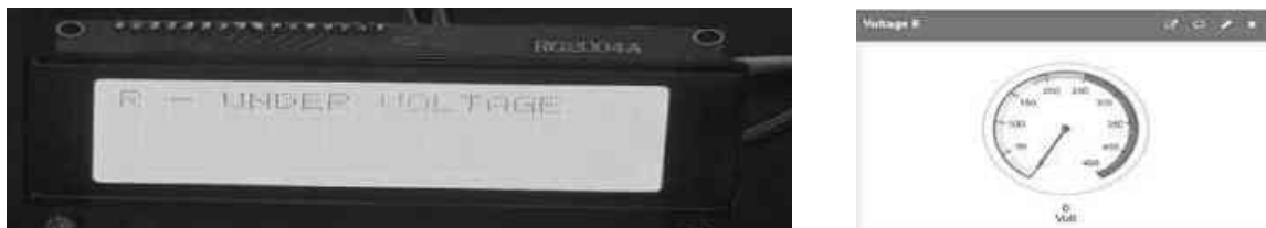
Figure 8: R phase Under Voltage Fault detection
