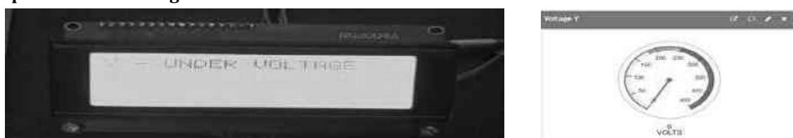
Figure 9: Y phase Under Voltage Fault detection
